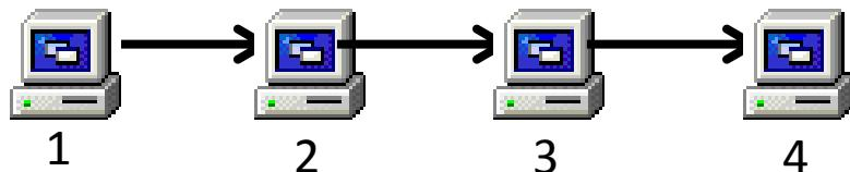
Transmission time of a single bit =  $\sum_{i=1}^n \frac{1}{C_i}$
