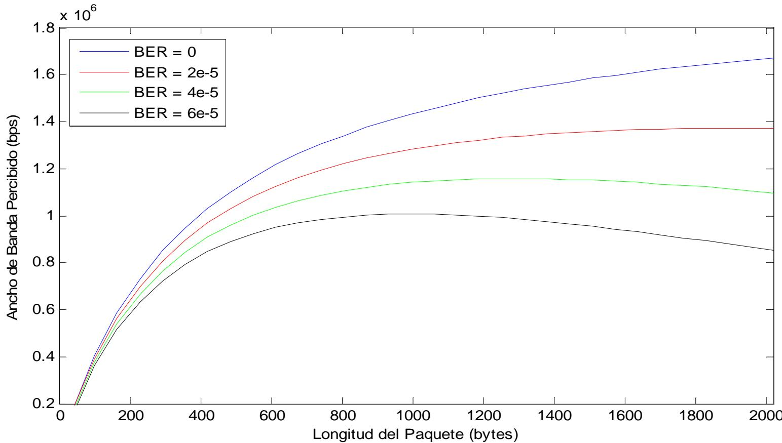
$$ABW(L) = a \frac{L}{\phi L + \delta} + (1-a)\gamma L \exp(-\lambda L)$$
