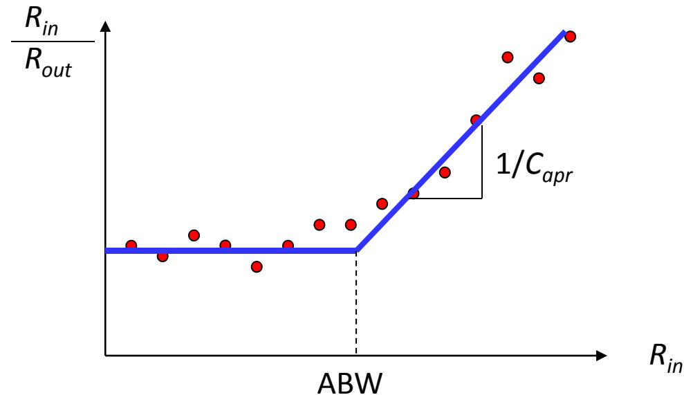
$$ABW(t-\tau, t) = \frac{1}{\tau} \int_{t-\tau}^t (C_{apr} - \lambda(s)) ds \stackrel{?}{=} \arg \max_R \left( R \middle| R + \frac{1}{\tau} \int_{t-\tau}^t \lambda(s) ds < C_{apr} \right)$$
