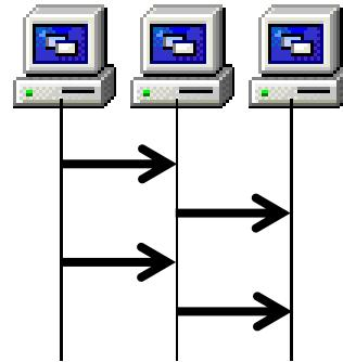
The gap between packets of the pair that have the minimum sum of OWD (SOWD) represents the effective time it takes a packet of the given length to get the destination.
