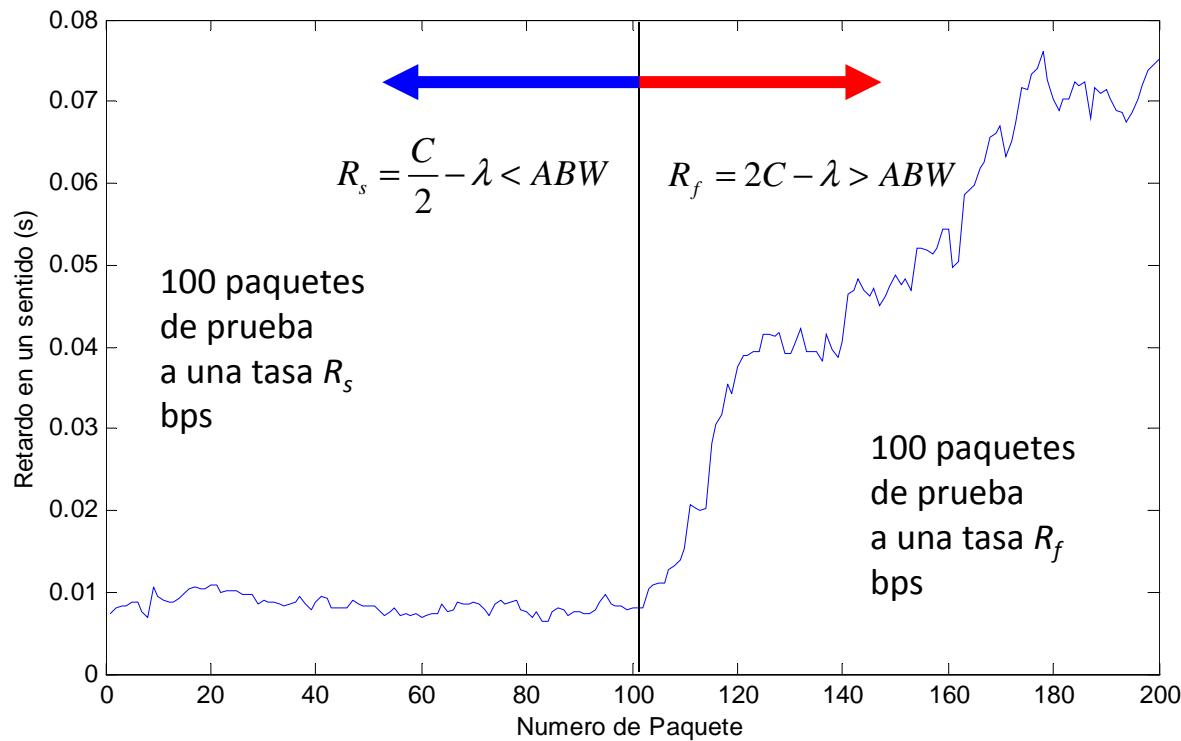
**SLoPS (Self Loading Periodic Stream)** : Tx sends a periodic flow of probing packets at a rate  $R$ . Rx measures the OWD of each probing packet and returns the tendency. Tx adjusts  $R$  in a binary search.
